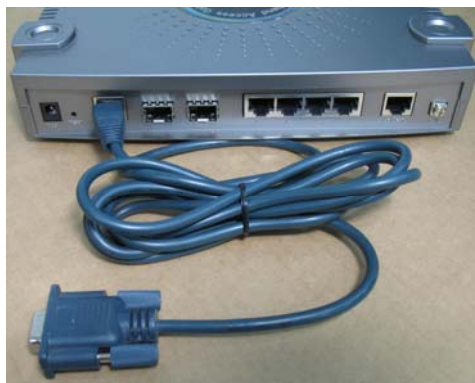
< Figure 3-6 > Console Cable Connected to N560 series
